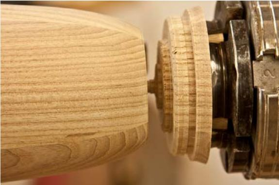
Once you finish sanding, using a parting tool part the vase ALMOST off. Be sure to make the bottom concave. Remove from the lathe cut off the nub, sand the bottom and finish the outside.
