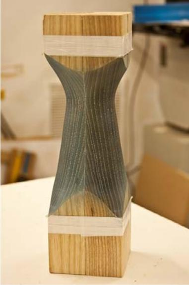
Do not finish the surfaces that are taped, this is where you will apply glue. Split the piece a part and rotate each square 180 degrees.
