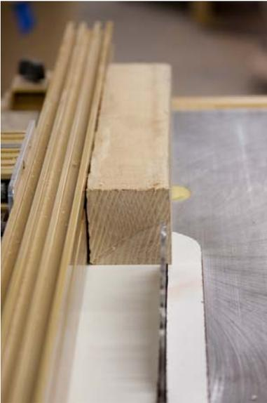
Without adjusting the fence and with the side that was marked against the table rip the piece again. Again keep the stock flat against the table and against the fence. The piece does not have to be square against the fence.
