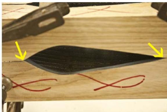
Make sure the corners indicated by the arrows are aligned correctly. If you only have four clamps wait a couple of hours after gluing squares 1 & 2 and 3 & 3, then glue the two halves together, making sure the corners are aligned. If you have 8 clamps you can glue the piece at one time.
