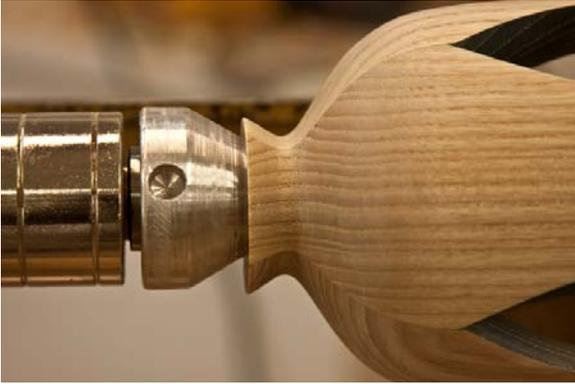
Put a cone on your live center to continue supporting the piece and turn the rim of the vase. Sand the piece. If you get any chip out on the edges of the openings hand sand them, feathering them. There should not be much if any chip out. Since this is basically a spindle, sanding on the lathe will most likely
