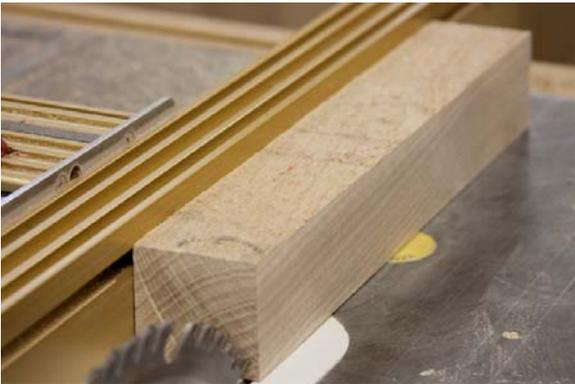
Set your fence to the final size of your stock. In this case 1-7/8 inches. With one of marked sides against the table and the other marked side against the fence, rip one side of the stock to the final size. The side against the fence should now be square with the fence. Flip the block 180 degrees
