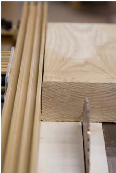
Square your stock using your table saw. (A band saw with a good quality  $1/2$  blade can be used, cutting is just a bit slower.) Make sure your blade is 90 degrees to the table of your saw. This is critical. Otherwise you will have a block that is a parallelogram instead of a square block.
