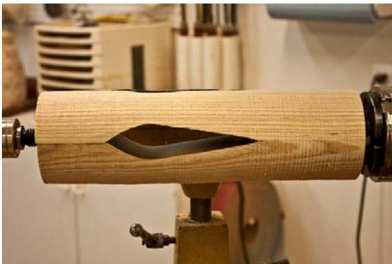
Once the glue has cured, mount the blank between centers and rough turn it round. On the bottom turn a tenon for your chuck. Mount in your chuck and bring the tail stock up for support.
