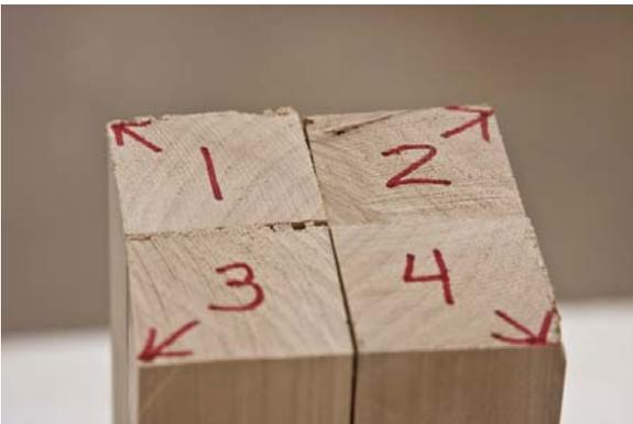
Arrange the blocks for the grain pattern you want for the outside of the piece. Number the blocks and mark the outside corners.
