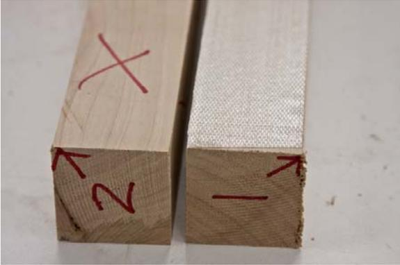
Rotate the pieces 180 degrees. Then using double sided indoor / outdoor carpet tape (the type with fiber glass threads) attach blocks 1 and two together
