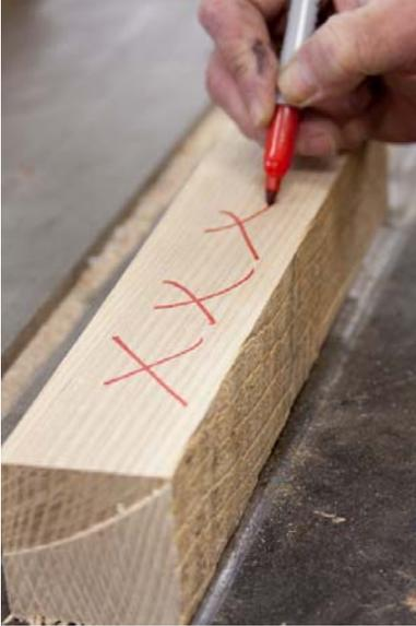
After ripping the first piece mark the edge that was just cut. This is a reference side for squaring. Repeat this procedure for the other three pieces.
