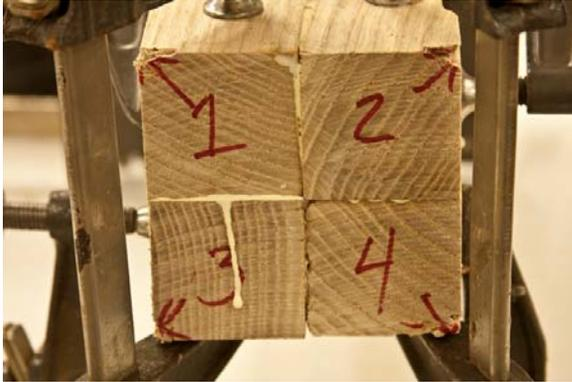
When the block is glued your numbers and aligning marks should look like this your original starting point. I let the glue dry over night to completely cure.
