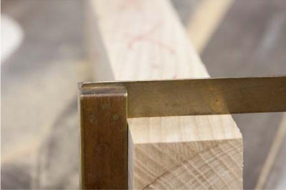
If your blade was set accurately to 90 degrees, the two sides that are marked should be square to each other.
