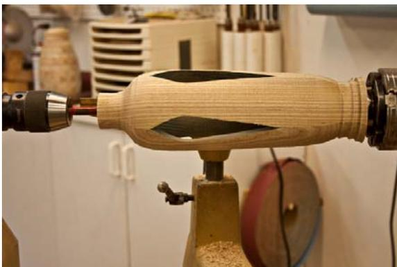
Using a 1 inch forstner bit in a Jacobs chuck drill a hole through the top. This will allow a 1 x 6 test tube to be inserted for flowers. The tube must have a “flared” top. They are available from Craft Supply part number 031-0300.
