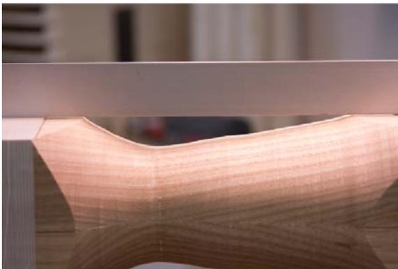
On this piece the smallest diameter is actually a little larger than 2-1/4 inches. If you want to see how the opening is going to look, lay a straight edge across the piece on flat edge (not on the corners). By checking as you are turning you can refine the opening to get the look you want. Once you are satisfied,
